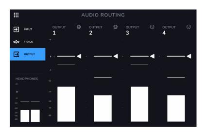
To adjust the output level of an individual output, tap and drag the white line at the top of its meter. Double-tap the meter to return the fader to the default **O dB** level.
