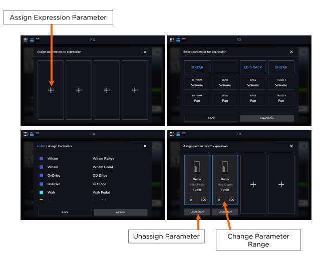
To assign a parameter to the expression pedal, tap the + sign in an empty slot, and then select an FX Rack, looper track volume or looper track panning parameter to assign.
