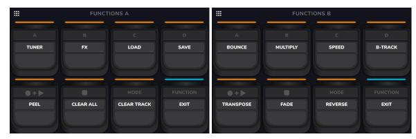
To select a function, press the corresponding **pedal** (labeled on the top panel in orange) or tap it on the **touchscreen**.
